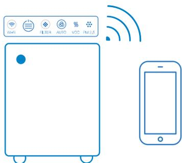
The air purifier can also be automatically regulated based on the air quality readings from the built-in sensors (480i), or the optional external air quality monitor Blueair Aware™ (405)
