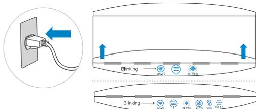
Open the flip-up lid and press the airflow speed touch button. When the Wi-Fi symbol starts to blink, the air purifier can be paired with the Blueair Friend mobile app.
